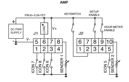
Resistive based sender input (i.e. temp, fuel and pressure).
