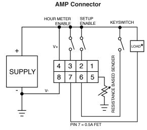
Resistive based sender input (i.e. temp, fuel and pressure).
