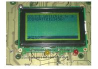
This menu enables to visualize the battery identification code set by the user with SW HFView. This field on the battery charger is not programmable, but requires use of SW HFView. P3 enables to exit the menu.
