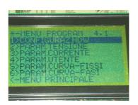
This menu enables to visualize and modify the battery charger parameters related to the charge curve.
