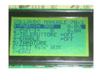
This window enables to execute a battery charger test, manually controlling certain signals managed by the CPU.
