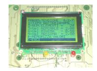
This menu enables to visualize and modify the parameters relative to battery type, number of cells, and nominal, minimum and maximum voltage.
