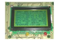
1<sup>st</sup> line: contains the battery charger size (for example 48V/40A) and the identification code of the charge curve and the ongoing phase (for example CURVE5-ph.01)
