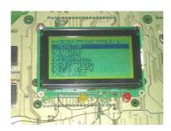
By pressing the buttons P1 and P2 one may select the desired sub-menu and press P3 to enter the selected menu.
