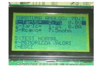
This window enables to execute circuit calibration to read analogue sizes, such as Voltage and battery current.
