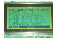
This menu enables to visualize and modify the parameters relative to the selected charge curve (among those present in storage (8 curves)), phase by phase (voltages, currents, Timer).
