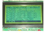
This menu enables to visualize and modify the parameters related to the curve currents and the set charge phase.
