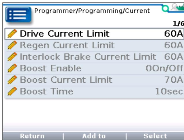
To edit a parameter with the 1313 Handheld Programmer, select the parameter:
