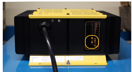
Figure 6: Bulk charge indicator displays charge profiles 7 and above.
