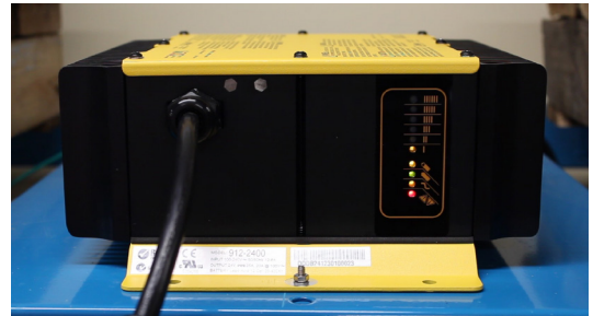
Figure 4: Charger LED indicator self-test.
