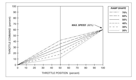
In all cases, the ramp shape number is the throttle command at half throttle. In Figure 12, for example, the 50% ramp shape results in a 30% throttle command at half throttle (i.e., a command that is halfway between 0% and 60%). The 20% ramp shape results in a 12% command at half throttle (20% of the range from 0% to 60%).
