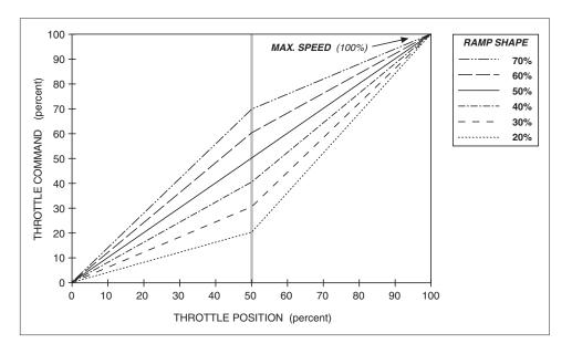
Changing the maximum speed setting changes the throttle command range, and hence the ramp shape. Ramp shapes with the maximum speed setting dropped from 100% to 60% are shown in Figure 12.
