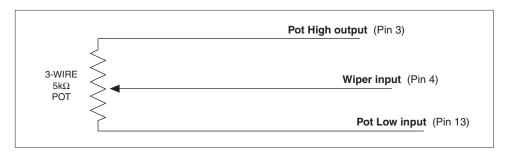
For wigwag and inverted wigwag applications, the pot can be correctly centered within the controller's neutral band by using the throttle autocalibration feature (see page 23). Pots with less than 5 k $\Omega$  total resistance change over the throttle's full stroke can be accommodated by programming the controller for reduced-range throttle inputs, via the throttle gain parameter (see page 25).
