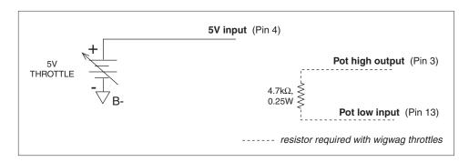
Voltage throttles with less than 5 V total voltage change over the full stroke can be accommodated by programming the controller for reduced-range throttle inputs, via the throttle gain parameter (see page 25).
