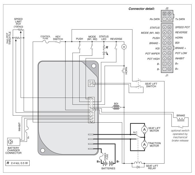
**Fig. 4b** Alternative wiring configuration, for low keyswitch current (≤ 9 A) applications with seat lift.
