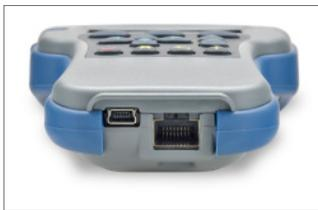
**USB Port** allows connection to PC for download of firmware and transfer of files.
