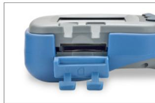
**SD Card Slot** for additional memory. SD card reader compatible with SD and SDHC. *SDXC not currently supported.*
