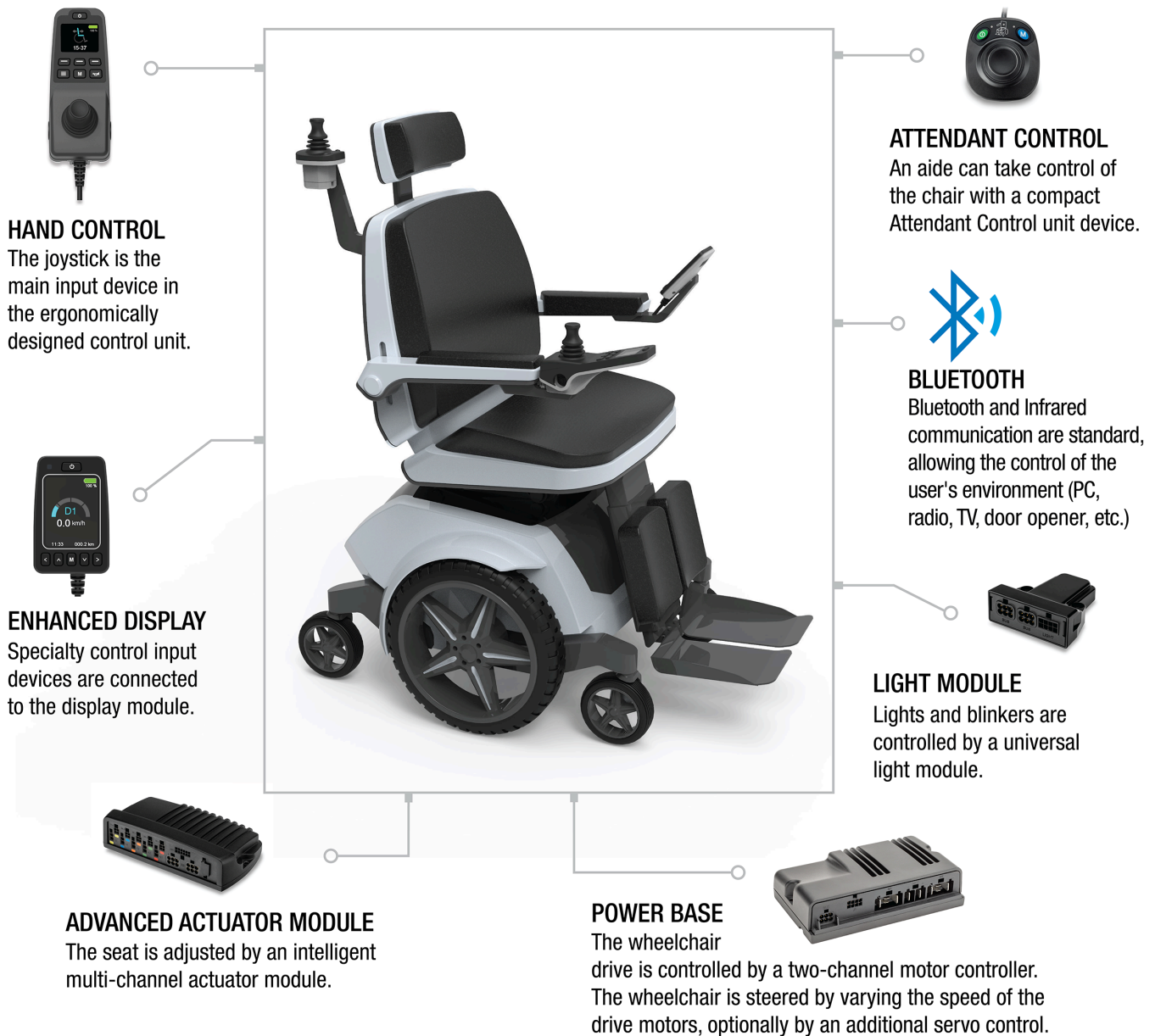
Figure 1. Wheelchair with the enAble® X1 System
