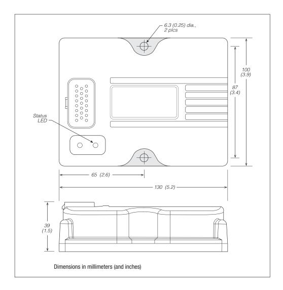
If the outputs will be used at or near their maximum ratings, it is recommended that the module be mounted to a good heatsinking surface, such as an aluminum plate.
