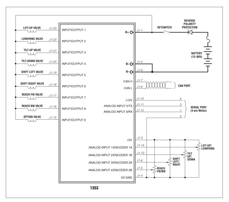
**Figure 4** *Application example, Curtis 1353 CANopen expansion module.*
