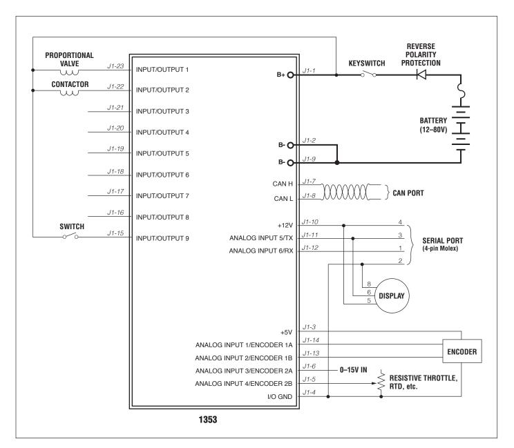
**Figure 3** *Basic wiring diagram, Curtis 1353 CANopen expansion module.*
