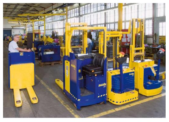
operated vehicles is a joint development based on Curtis's TH series. Due to the large rocker switches for the driving functions and an emergency reverse switch, it offers good ergonomics and maximum safety.
